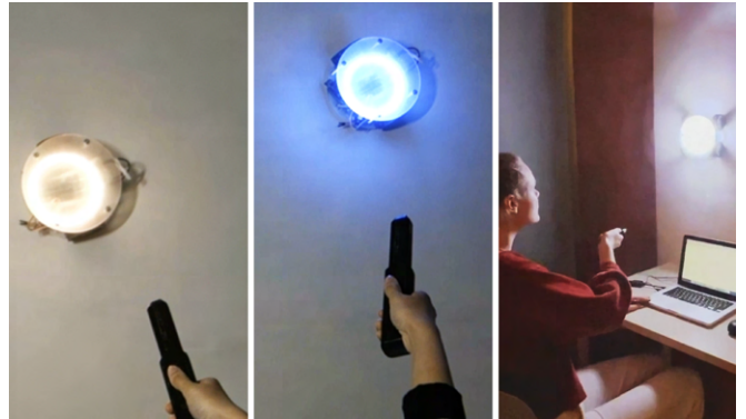
Fig. 1. Light Everywhere , a robotic lighting fixture that traverses walls and ceilings, user controlled for position, lighting mode, and lighting coverage.
