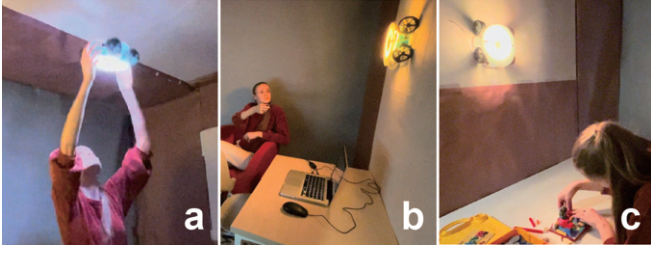
Fig. 6. The prototype functions: (a) being manually moved across surfaces; (b) climbing wall and ceiling surfaces, controlled via a remote; and (c) changing lighting modes between “white,” “yellow,” and “dim.”
